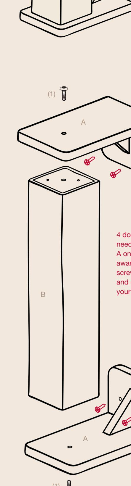
4 dowels and screws are needed to fix it with detail
